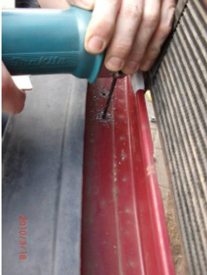
Pic. 3: holes in lower front body
